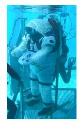
To be able to exist in the hostile environment of space, astronauts have to carry heavy and bulky space suits. Even under zero gravity conditions, these suits significantly restrain natural human manoeuvrability and dexterity. Procedures and technical systems enabling future human, or human-robot, space missions must be tested on earth using realistic space suit mock-ups.
