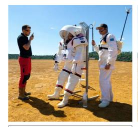
Mobile suitport: Steel frame for astronaut change in the field. Used to dock astronaut and release him/her from the weight of the suit at any time in case of emergency
