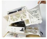
The Pantograph Sampling Tool is designed to facilitate easy collection of sample material. It allows the single-handed extension and contraction of a tool arm. The head of the tool serves as a shovel and at the same time, a sampling container with a closable lid. With a simple mechanism the container can be released and a new sample box can be affixed to the tool head. Samples are stored independently from one another to avoid cross-contamination.
