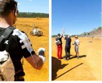
Gesture Control is a novel, yet intuitive, way to control and interact with robots. In contrast to most other control approaches, MOONWALK gesture control enables the user to perform true, hands-free control of the robot. It does not require the handling of any additional input devices, thus allowing for the simultaneous execution of different tasks (e.g. sampling), while controlling the robot.
