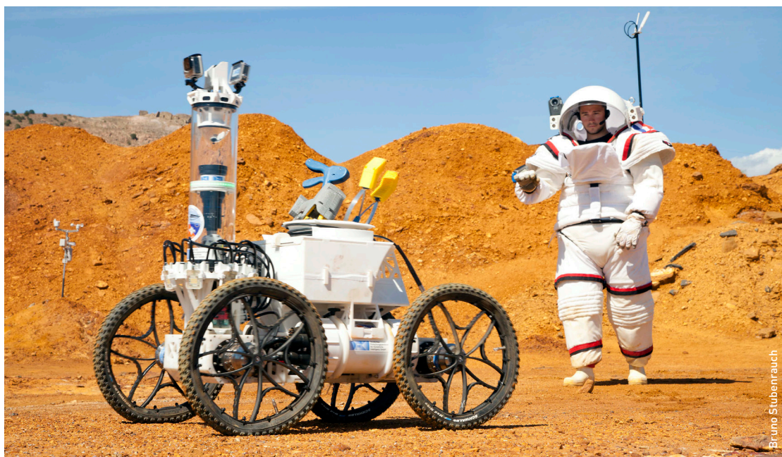
◀ Simulation astronaut gesture controls the rover on a Martian exploration simulation.
